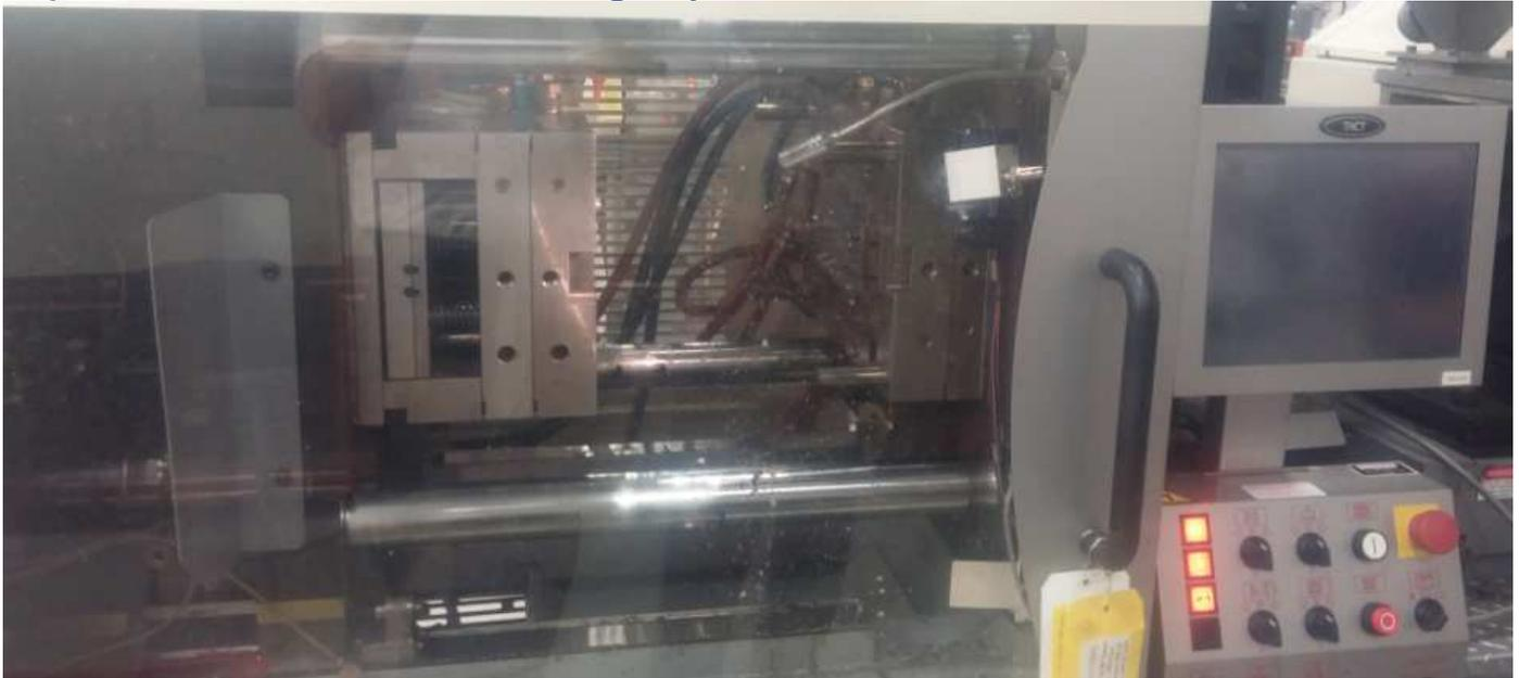
Process Sensors IR custom engineered, turn-key PSC-160 IMMS MoldMinder, interfaces seamlessly with injection mold machines.
